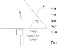
For squaring up a new fence, foundation, deck, or anything else that needs to be square, use the 3-4-5 rule. The best place to start is in one corner of the layout. The corner should be a right angle with two legs. The end of the left leg is A, the corner is B, and the end of the right leg is C. Tie a string between A and B to create left leg A, and tie a string between B and C to create right leg C. B is the corner.
