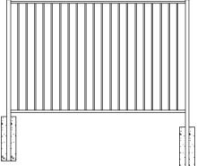
"Option #1"Now take a measurement On Center to determine where to pre drill 1/8" Diameter pilot hole so you can mark the rest of the post.
